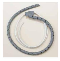
"Twist Tape" is a pre-formed Flexible Heater to fit piping from .25" Dia to 4.0". It is flexible and uniquely designed to accomplish those hard-to-fit requirements on a semi-permanent basis. Power-In-Power-Out leads allow for a parallel daisy chain installation.
